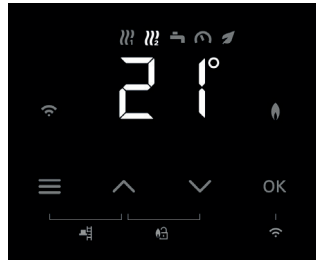
LCD screen with 7-segment display and touch buttons
